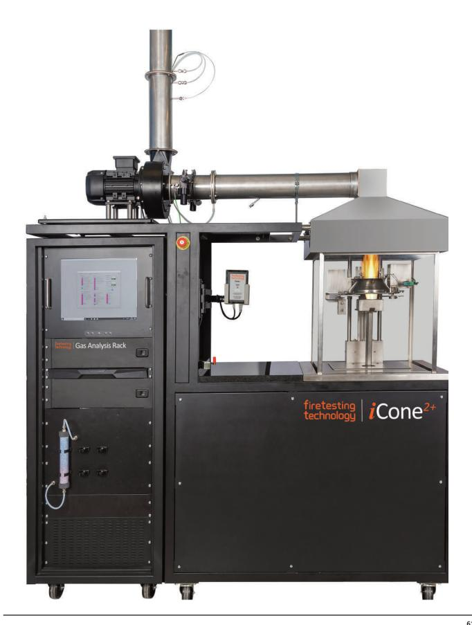
The *i*Cone<sup>2+</sup> is the latest development in the FTT *i*Cone range and incorporates all of the best features of our range of cone calorimeters. It offers cutting edge PCB based technology in a modular and robust build with remote communication, cone operation and diagnostic facilities that allow **FTT** the capability to efficiently respond, diagnose problems and service installations, in all corners of the world.
