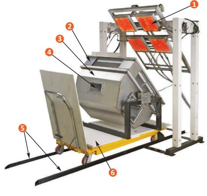
the Sample Trolley can be adjusted. The Sample Alignment Jig and a system of Stops are provided to reach the correct position.
