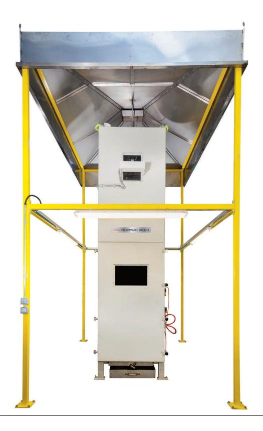
Heat release and smoke production measurement on cables during flame spread test. (Test apparatus also meets IEC 60332-3 series tests specification)
