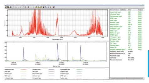
1000ppm. PAS will automatically switch and use the most suitable model for the current concentration mix.
