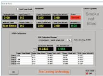
The software interfaces with the OSU apparatus via a data logger system, into which all the required signals are connected
