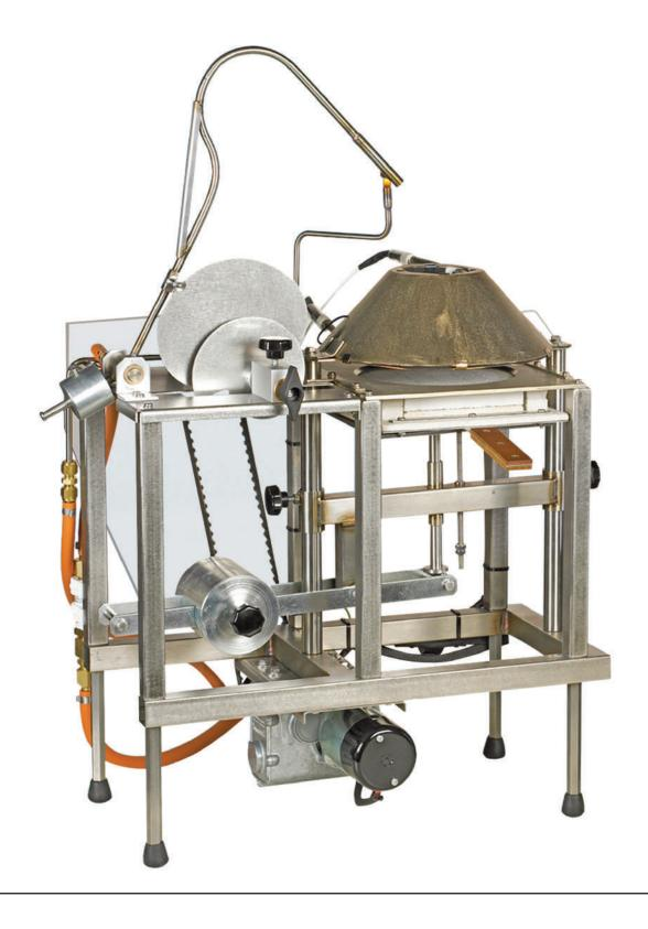
ISO 5657, BS 476 Part 13: Ignitability of building products using a radiant heat source The capability of a material to be ignited is a critical property to measure and is a highly important element in any assessment of fire hazard.
