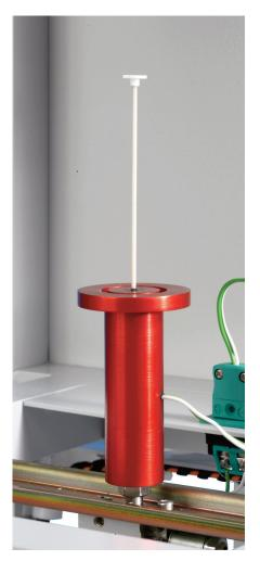
The FTT Micro Calorimeter was developed in co-operation with the Federal Aviation Administration (FAA). It determines fundamental thermo-chemical data in seconds and predicts fire properties of materials.
