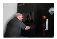
Instrument access via airtight gauntlets and viewing panel
