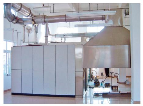
Figure 2: FTT ISO 9705-2 Large Scale Calorimeter with Weight Measurement (Room chamber on left not included in standard configuration) Courtesy from the Shanghal Fire Research Institute
