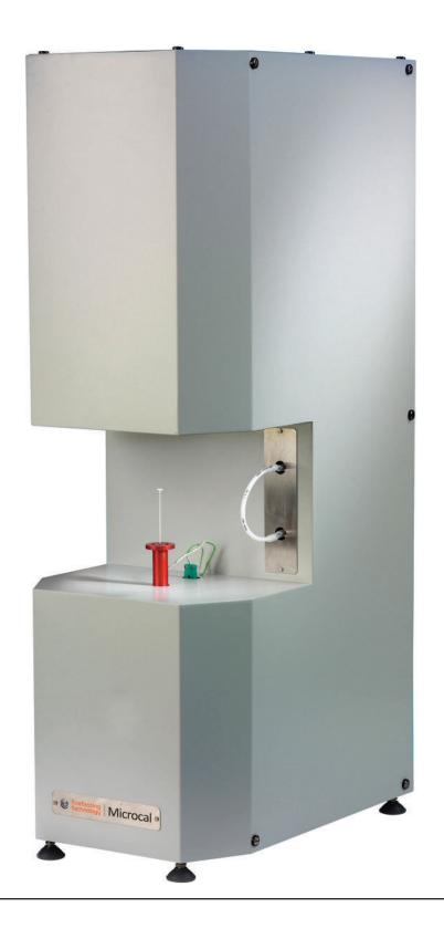
Accurate and cost effective micro calorimetry using a Pyrolysis Combustion Flow Calorimeter (PCFC) ASTM D7309
