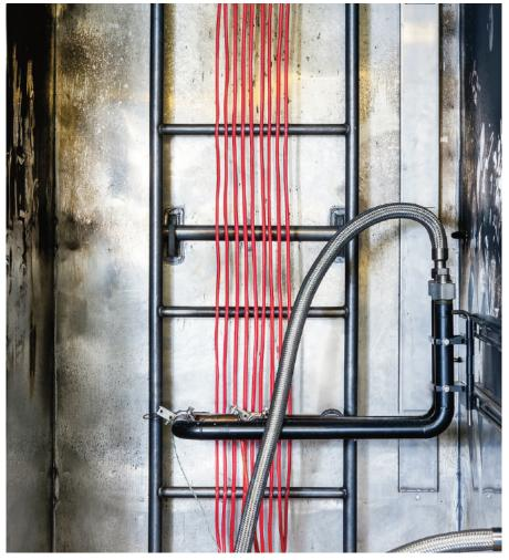
Test chamber interior detail with propane burner
