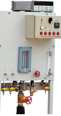
Gas Panel, Control Box and Data Logger
