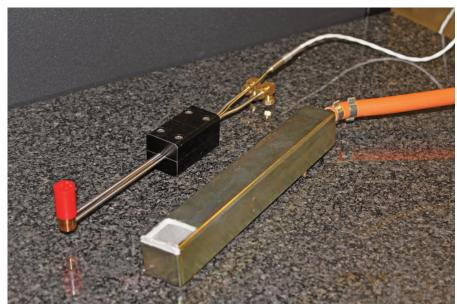
Heat flux meter and calibration burner
