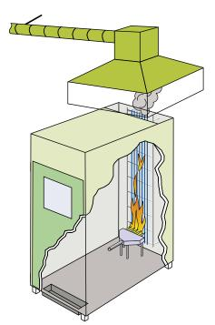
Figure 10: FTT EN 60332-3 Vertical Flame Propagation Test for vertically mounted bunched cables
