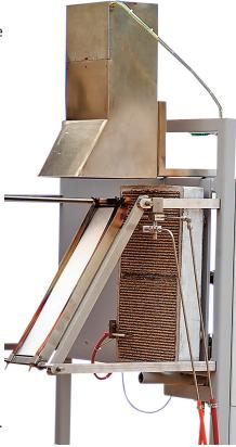
Radiant Panel, Specimen Holder and Exhaust Stack
