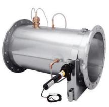
Duct section placed in EN 50399 exhaust
