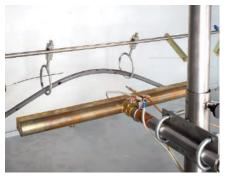
Ring Clamps for Resistance to Fire Alone Testing
