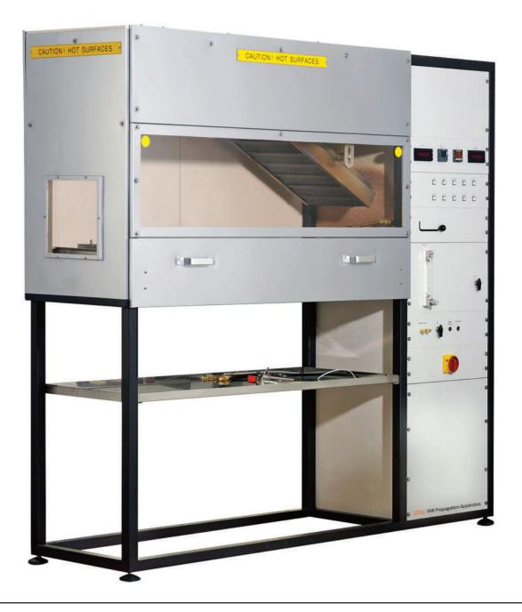
This test method is used to evaluate the flammability and flame propagation characteristics of thermal/acoustic insulation when exposed to both a radiant heat source and flame in a test chamber.
