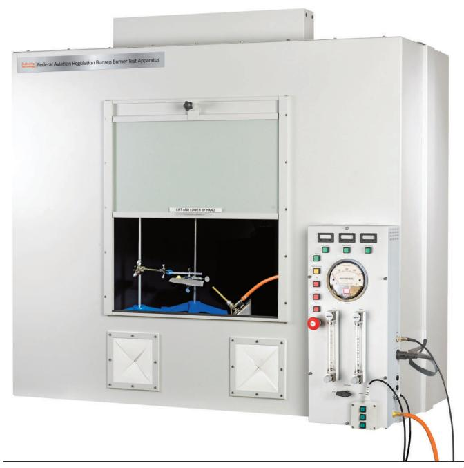
The FTT Federal Aviation Authority (FAA) Bunsen Burner Test Apparatus conforms to the fire test methods described in FAA Aircraft Material Fire Test Handbook for aircraft materials. The apparatus is supplied as a complete system incorporating all the features necessary for ease of use and safety. It enables the user to test according to five Federal Aviation Regulation (FAR) test methods. These are:
