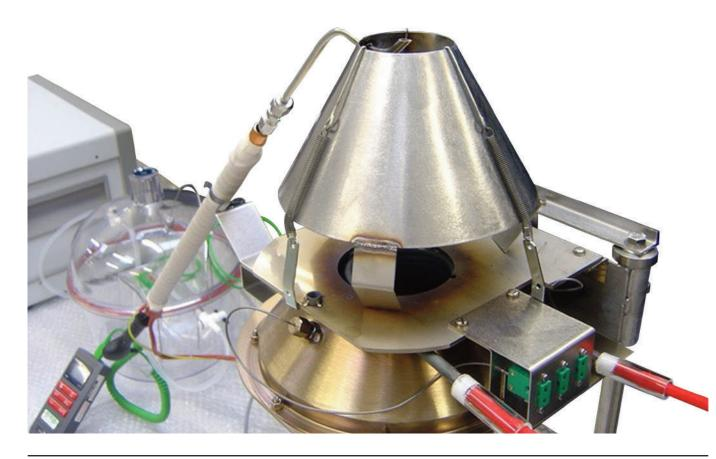
The Cone Calorimeter and Mass Loss Calorimeter can be used to determine the corrosive effect of combustion products when used with a cone corrosimeter.
