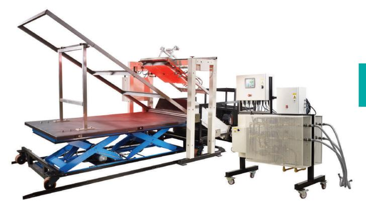
This ENV 1187 describes four methods for determining the performance of roofs to external fire exposure. The four methods assess the performance of roofs under the following condition
