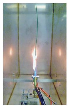
Figure 9: FTT EN 60332-1 Flame Propagation Test for a Single Wire or Cable
