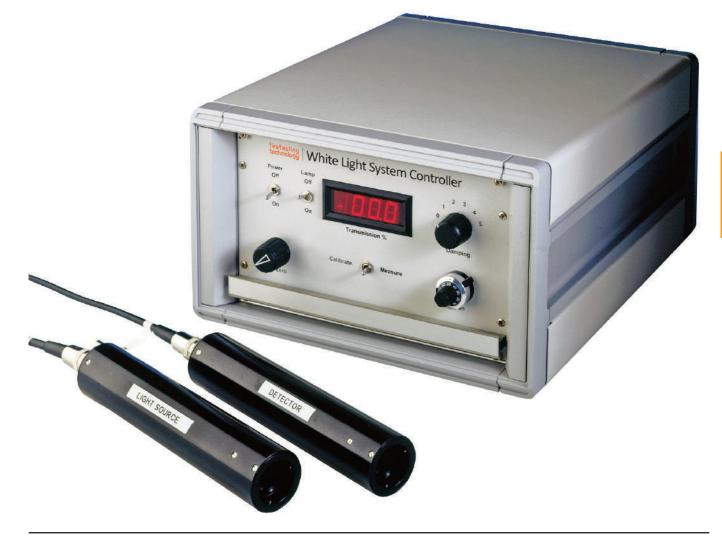
The FTT 'Smoke Density Photometric System' (DIN 50055) is designed to be used in conjunction with equipment that measures smoke from burning materials. The unit can be fitted to several instruments such as the Room Corner test, (ISO 9705), Single Burning Item (SBI) (EN 13823), Heat Release and Smoke Production Apparatus for IEC 60332 Part 3 (EN 50339), Steiner Tunnel (ASTM E84) or Flooring Radiant Panel (EN 9239-1) etc.
