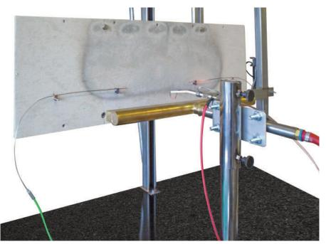
**Resistance to Fire with Mechanical Shock**
